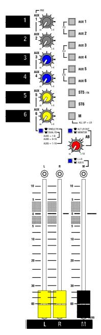
**AUX MASTERS** Each aux mix has a master level control that adjusts the output level to match external equipment, or to trim the monitor, effect or other send without affecting the mix balance. Up to +4dB boost is available above the normal 0dB position.
